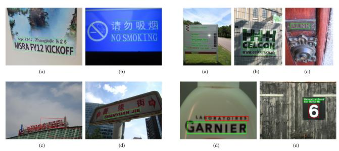
Figure 8. Detection examples of our model on MSRA-TD500. (a)-(b) Chinese text can also be detected due to the model generalization. (c)-(d) Some failure cases for complicated background or wide character space. False and miss detected texts are enclosed by red lines.
