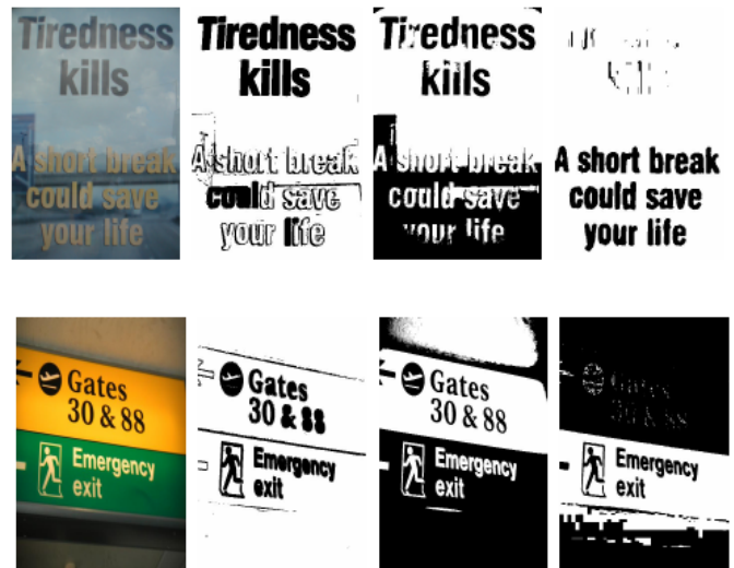
Fig. 3. Multi-level binarization results of two test images. From left-to-right images are shown followed by their binarization results for: smooth/non-smooth binarization, adaptive thresholding binarization on the original image and on the complement of the Hue channel. Note that some text components appear in only one of the binary image.
