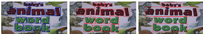
Fig. 7. Left: original image with all the text components. Middle: output of the first grouping step: the resulting boxes are mostly letters (or few merged letters merged). Right: final grouping output: text grouped at word level.
