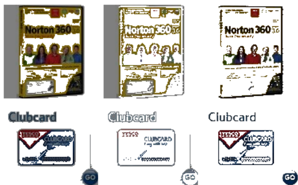
Fig. 4. Text pixels and adjacent non-text pixels are separated by binarization. Left: regions isolated by white pixels. Middle: image L with low-value CCs. Right: image H with high-value CCs.
