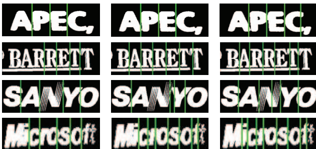
Figure 3. Representative segmentation results of different methods. Left: ContourSeg, Middle: GraySeg, Right: Our method.
